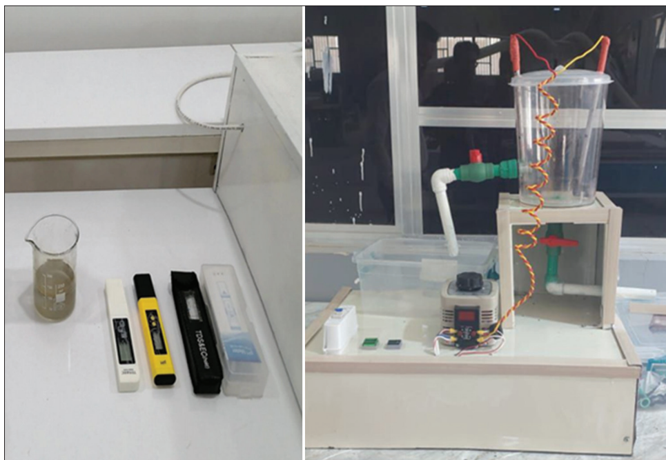
Figure 3: Locally manufactured electro-Fenton device for the experiment.
